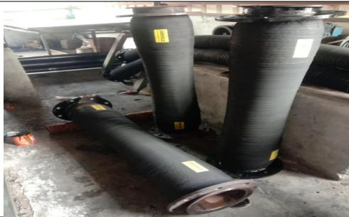
SANDHYAFLE X-125NB-CFRH 5" (125mm)I D x 5Mtr (LG)
